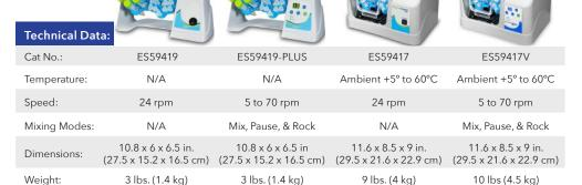
Our Roto-Therm series of rotating mixers provide a wide range of mixing capabilities. Suitable for an array of laboratory applications including resuspension, protein binding, nucleic acid purification, histochemistry, hybridization etc, the mixers include interchangeable tube holders for accommodating all common tube sizes from 0.5mL to 50mL. The motion can be adjusted from vertical (end over end) mixing, to horizontal (rolling or hybridization style) mixing.
